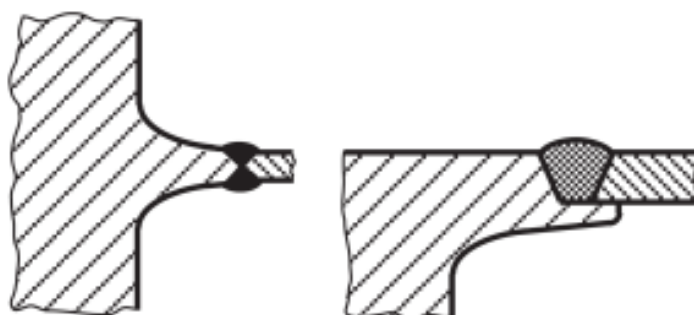
Fig. C3.6.2 Welding flanges on steel castings or forgings
